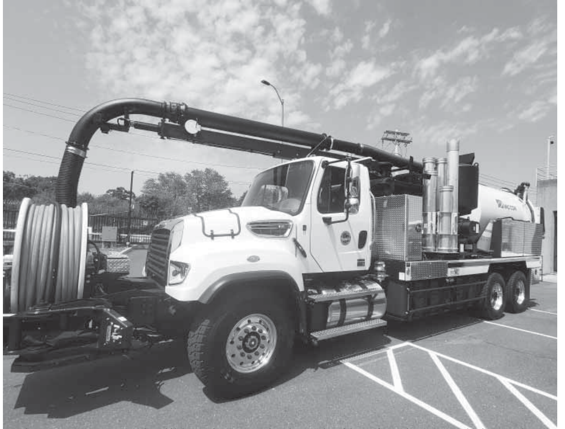
The new vacuum truck will help city crews in the task of keeping city storm drains and sewer lines free from debris.
